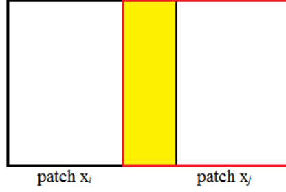
Figure 3.5: The patch-patch compatibility function is computed from the sum of squared pixel differences in the overlap region.
