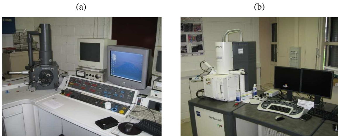
Fig. 4.4 Scanning Electron Microscope (SEM) equipped with EBSD system: (a) Cambridge S360 (W-GUN) and (b) Zeiss Supra 40VP used in our experiments (LSPM laboratory, University Paris 13).
