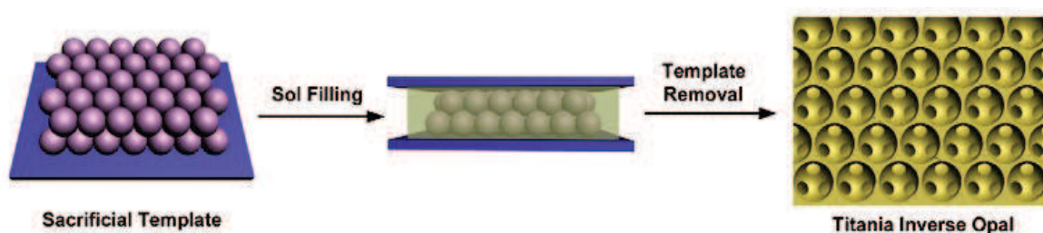
Figure 9: Schematic fabrication process for the formation of titania inverse opal by an optimized sol-gel opal infiltration. [20]
