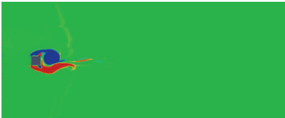
Figure 4.35: Vorticity flow past a rectangle. Solution at instant T = 10s computed with the 2 level SWR implicit scheme. The unit square is closer to the border, at position [2, -.5] .
