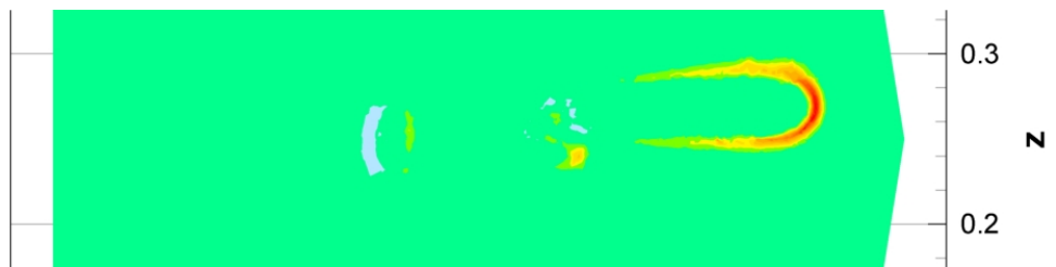
Figure 6.30: Net charge density at times t_1 = 1.89 \cdot 10^{-8} s, isolines in a cut plane y = 0.25
