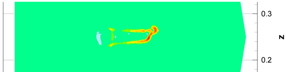
Figure 6.27: Net charge density at times t_1 = 1.31 \cdot 10^{-8} s, isolines in a cut plane y = 0.25
