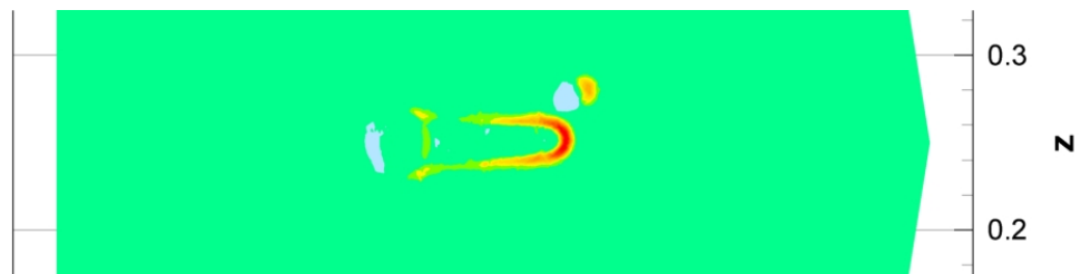
Figure 6.96: Net charge density at times t_1 = 1.31 \cdot 10^{-8} s, isolines in a cut plane y = 0.25
