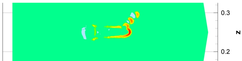
Figure 6.72: Net charge density at times t_1 = 1.36 \cdot 10^{-8} s, isolines in a cut plane y = 0.25
