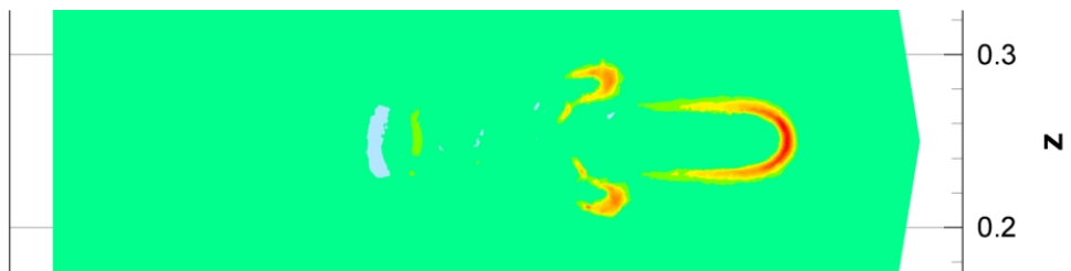
Figure 6.100: Net charge density at times t_1 = 1.89 \cdot 10^{-8} s, isolines in a cut plane y = 0.25
