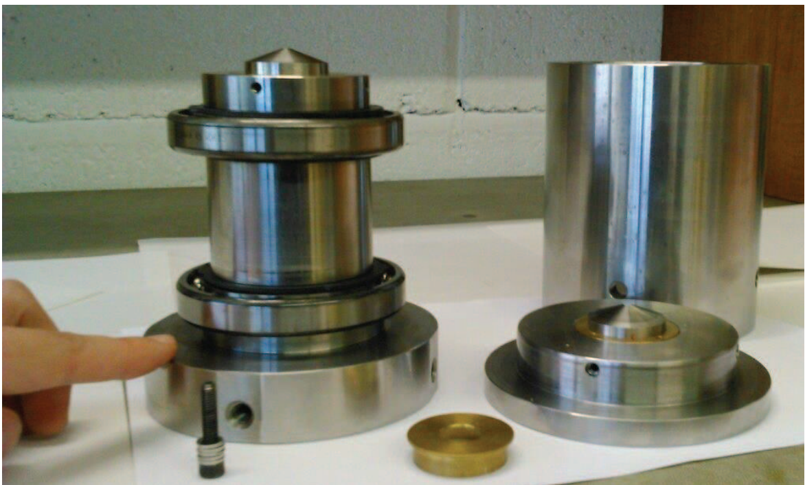
Figure II.12 Photo of high pressure system equipped with pair of Bridgman anvils.
