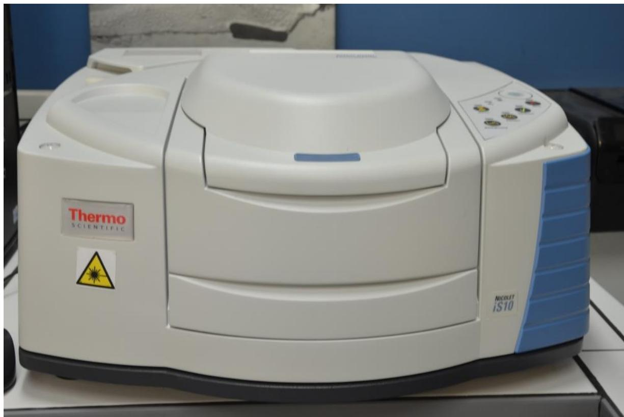
**Figure 34: Nicolet IS10 FT-IR Spectrometer**
