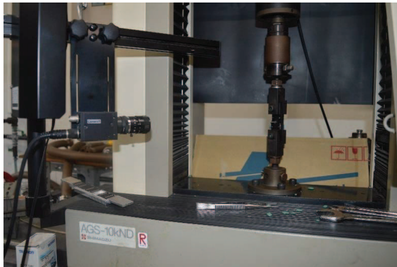
Figure 4-12 : Machine de traction Shimadzu AGS-10kND
