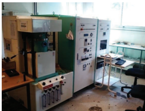
Figure 2-16: Dispositif SPS de l'ICMPE (Thiais, France)
