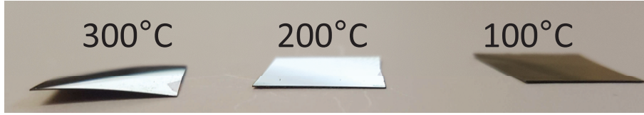
Figure 6.2.4 – Photography of three CFB samples annealed at different temperature (100°C, 200°C and 300°C) showing increasing cylindrical bending with annealing temperature. .
