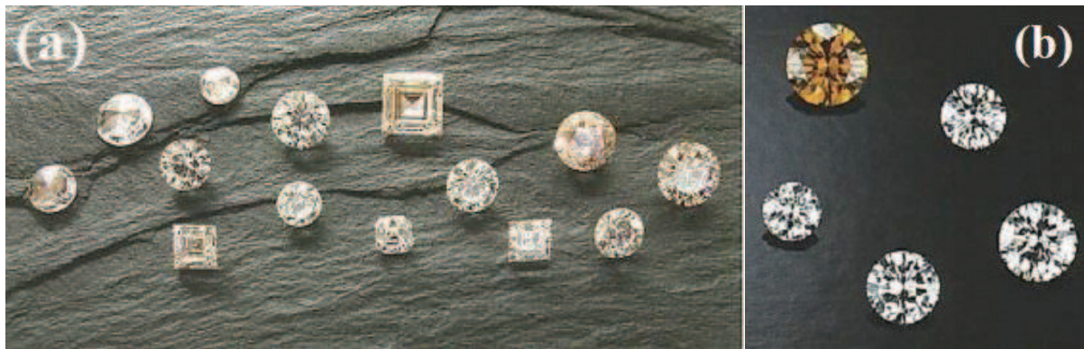
Figure I.3. Diamond single crystals of gemmological quality and different colour cut in jewel form are reported. (a) The synthesis techniques of productions are CVD by Element6 (from 0.21 to 1.04 carats) [19] and (b) HPHT by De Beers [20].
