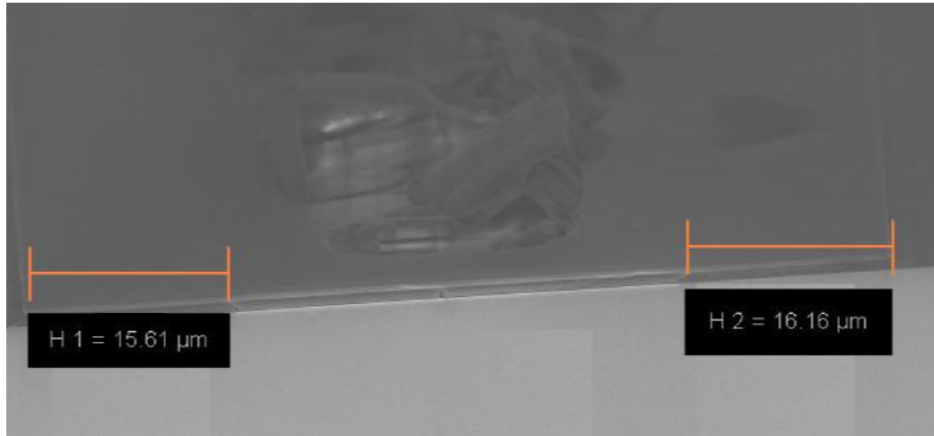
Figure 37: SEM image of a 70\mu\text{m} wide waveguide. After oxidation at 410\text{ }^\circ\text{C} for 1h, it was left in contact with air for 1 month. Severe surface delamination is present in the unoxidised central zone.
