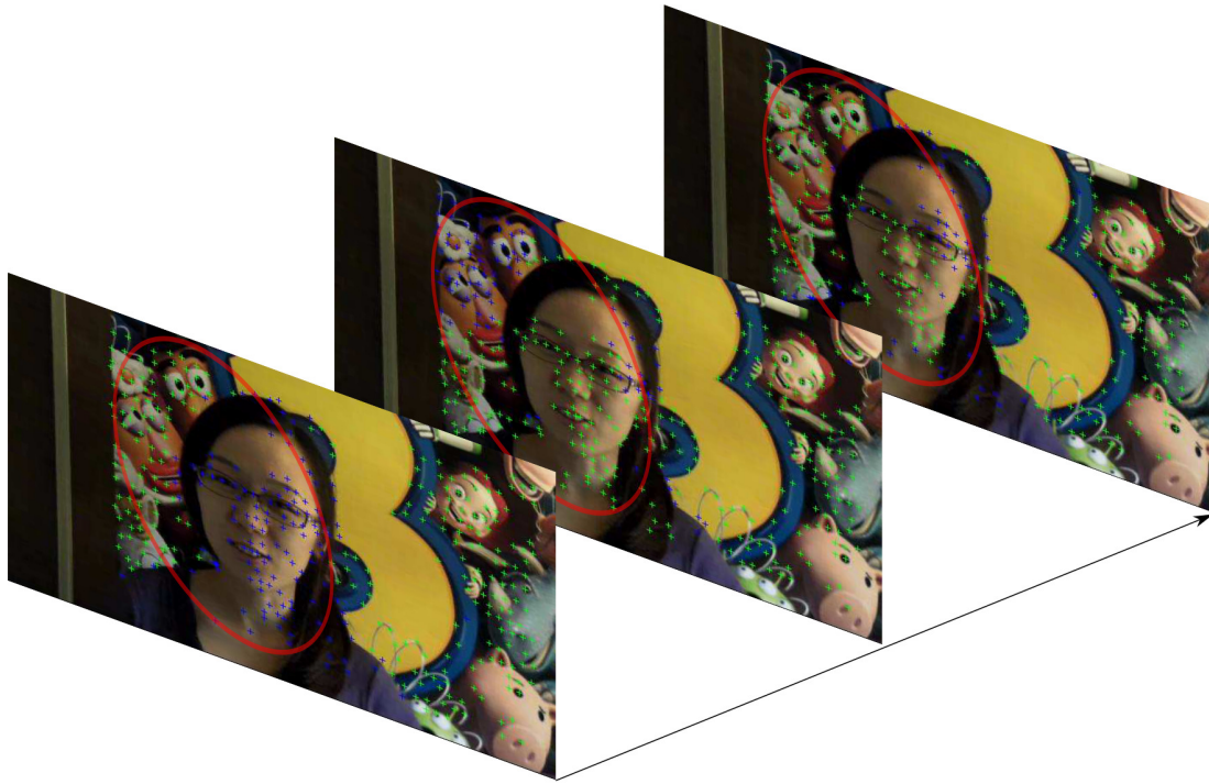
Figure 4.2 Three successive frames from the close_person sequence. Feature points classified as inliers by RANSAC are marked in green, while feature points classified as outliers are marked in blue. In the area circled in red, we can see that most feature points located on the person or in upper left corner change status abruptly.
