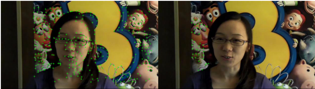
Figure 4.8 Example on the close_person video (frame 100). On the left frame are all trajectories detected by the KLT tracker, and on the right are the selected trajectories. All trajectories corresponding to the moving woman have been removed.
