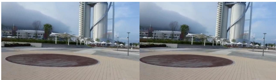
Figure 1.6 Illustration of the rolling shutter effect. Note the tilted tower in the second frame. This is caused by fast camera movements from left to right, which causes vertical edges to be seen as diagonal as the camera changes position between capturing successive rows.
