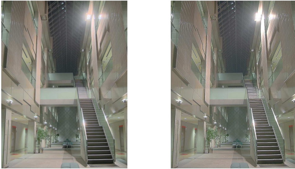
Figure 5.19: "AtriumNight" HDR test image (28.68 f-stops) - Left image: Pro_CEDP_Opt_L1_N1 (TMQI1=0.806); Right image: Pro_SEPENOCA_L1 (TMQI1=0.973).
