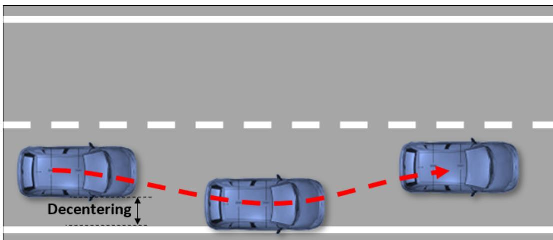
**Figure 3.8.** : Use case illustration : Ego drifts from its lane and cross the white line on the side of the road, before being put back in the runway center
