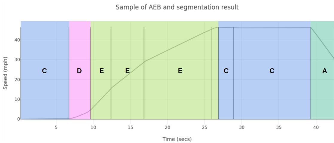
**Figure 2.3.** : Segment sequence encoded using the dictionary. Two stationary patterns can be recognized (b and c), corresponding to cruise speed phases, as well as two accelerating (d and e) and one decelerating (a).
