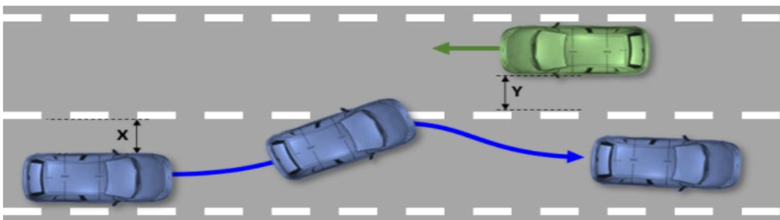
**Figure 4.4.** : Use case illustration : ego drifts from its lane, crosses the center line and heads toward an oncoming vehicle. The system detects the target and change ego's direction.
