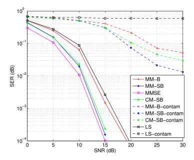
Figure 3.12: SER vs SNR with pilot contamination ( $N_c=3$ ,  $N_t=2$ ) (MIMO-OFDM model).
