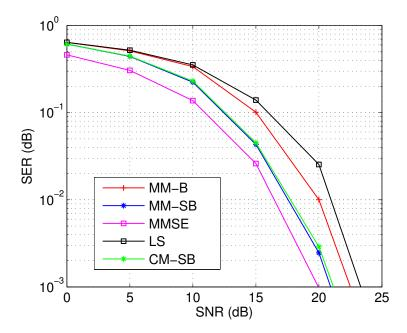
Figure 3.7: SER vs SNR with LS (MIMO-OFDM model).
