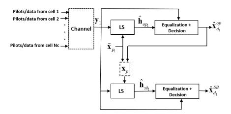
Figure 2.4: LS-DF semi-blind channel estimation approach.
