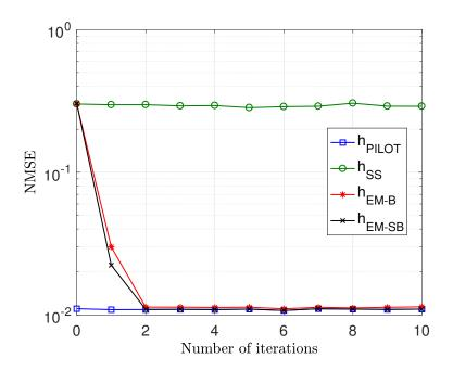
**Figure 5.12:** NMSE vs. number of iterations for subspace-based estimator  $(h_{SS})$ , blind  $(h_{EM-B})$  and semi-blind  $(h_{EM-SB})$  EM-based estimators benchmarked against the fully-pilot-based estimator  $(h_{PILOT})$ , in the case of a quadratic model and 4-QAM modulation at SNR = 10 dB.
