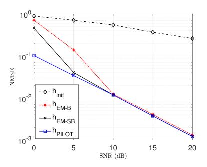
**Figure 5.6:** NMSE vs. SNR for blind  $(h_{EM-B})$  and semi-blind  $(h_{EM-SB})$  EM-based estimators benchmarked against the fully-pilot-based estimator  $(h_{PILOT})$ . We consider a quadratic model, 4-QAM modulation and a MIMO system with  $N_t = 2, N_r = 4$ , and M = 2.  $h_{init}$  is included for reference and refers to a pilot-based estimator using available pilot symbols.
