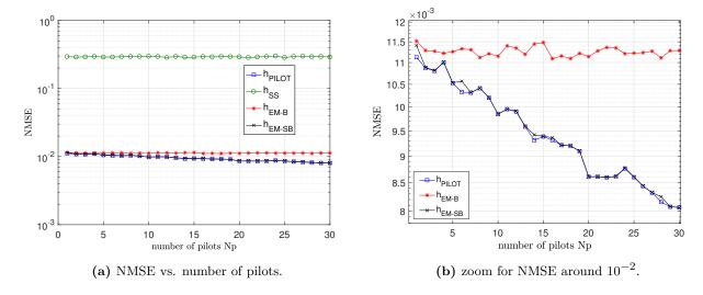
Figure 5.13: NMSE vs. number of pilots  $N_p$  for subspace-based estimator  $(h_{SS})$ , blind  $(h_{EM-B})$  and semi-blind  $(h_{EM-SB})$  EM-based estimators benchmarked against the fully-pilot-based estimator  $(h_{PILOT})$ , with a quadratic model and 4-QAM modulation at SNR = 10 dB.
