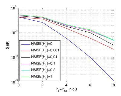
Figure 6.5: SER vs. power level between linear and nonlinear terms  $P_L - P_{NL}$ , with variable linear channel estimate accuracy  $NMSE(H_L)$  at SNR = 10dB.
