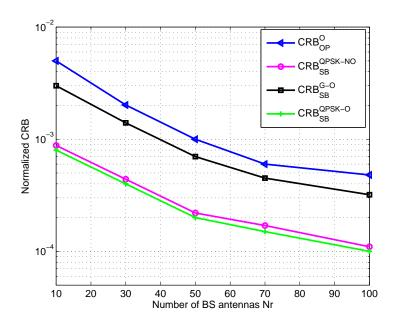
Figure 2.10: Normalized CRB versus number of BS antennas  $N_r$ .
