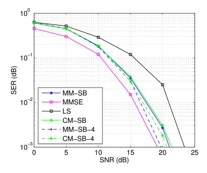
Figure 3.8: SER vs SNR with LF (MIMO-OFDM model).
