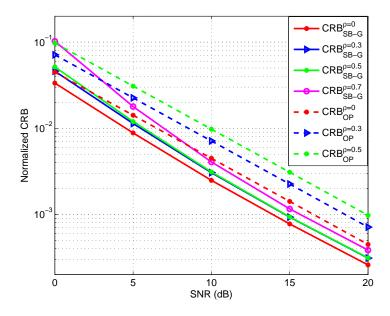
Figure 2.7: Gaussian CRB versus SNR with different orthogonality levels.
