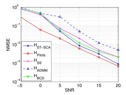
Figure 4.1: NMSE of channel matrix H estimate vs. SNR.
