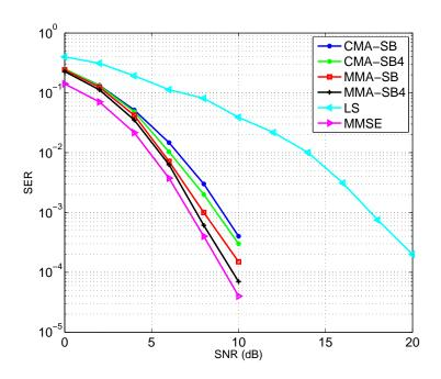
Figure 3.3: Average SER vs SNR with LS and LF  $(N_r = 20, N_t = 4, N_d = 100, N_p = 5)$
