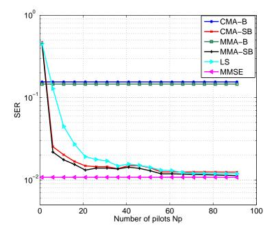
Figure 3.4: Average SER vs number of pilots  $N_p$  for blind and semi-blind source separation ( $N_r = 20, N_t = 4, N_d = 100, SNR = 5dB$ )
