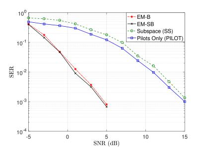
**Figure 5.14:** SER vs. SNR for subspace-based estimator (SS), blind (EM-B) and semi-blind (EM-SB) EM-based estimators benchmarked against the fully-pilot-based estimator (PILOT), with a quadratic model and 4-QAM modulation.
