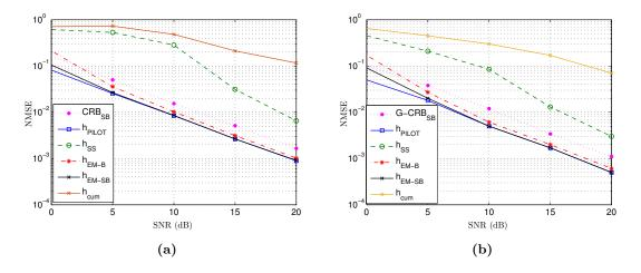
**Figure 5.5:** NMSE vs. SNR for subspace-based estimator  $(h_{SS})$ , blind  $(h_{EM-B})$  and semi-blind  $(h_{EM-SB})$  EM-based estimators benchmarked against the semi-blind Gaussian CRB (G-CRB<sub>SB</sub>), the cumulant-based technique [1]  $(h_{cum})$  and the fully-pilot-based estimator  $(h_{PILOT})$ , in both cases: (a) quadratic model and 4-QAM modulation, and (b) quadratic model and 16-QAM modulation.
