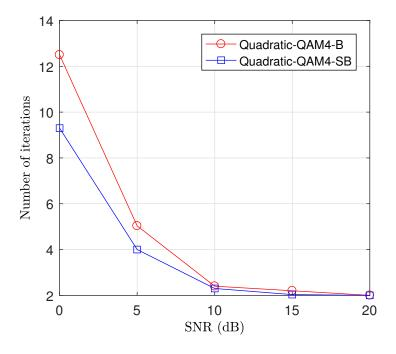
**Figure 5.11:** Number of iterations for convergence vs. SNR considering a quadratic model, a 4-QAM modulation, and  $N_r = 9$  receive antennas.
