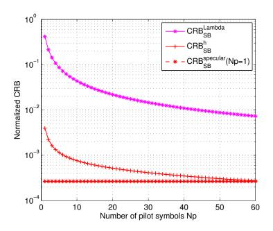
Figure A.2: Normalized CRB vs number of pilot symbols.
