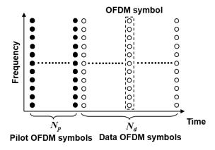
Figure 2.3: Block-type pilot arrangement
