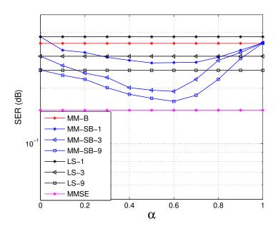
Figure 3.11: SER vs  $\alpha$  with Np = 1,3,9 pilot symbols (MIMO-OFDM model).
