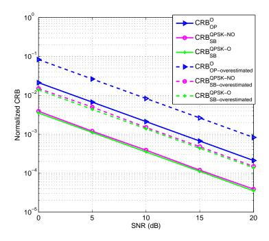
Figure 2.11: Normalized CRB versus SNR with channel order overestimation.
