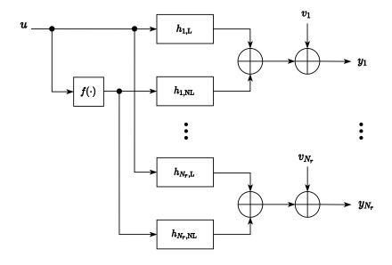
**Figure 5.2:** Architecture of the considered SIMO system, where f(.) is a nonlinear function w.r.t. the linear signal  ${\bf u}$
