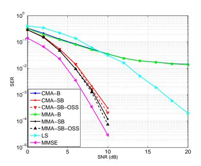
Figure 3.1: Average SER vs SNR for blind and semi-blind source separation with random initialization  $(N_r = 20, N_t = 4, N_d = 100, N_p = 5)$
