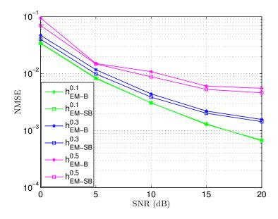
**Figure 5.3:** NMSE vs. SNR with different values of the weight  $\alpha$  (see (5.48)), indicated in superscript, for the blind and semi-blind 'linear' EM-based estimators.
