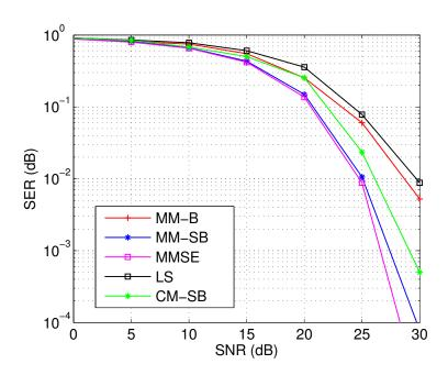
Figure 3.9:  $SER\ vs\ SNR\ with\ 16\mbox{-}QAM\ (MIMO\mbox{-}OFDM\ model).$
