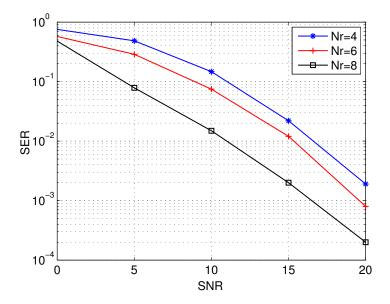
Figure 6.6: SER v.s. SNR for different number of receive antennas  $N_r$ .
