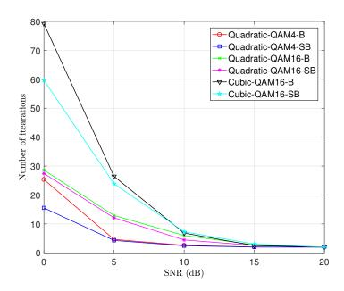
**Figure 5.10:** Number of iterations for convergence vs. SNR for blind (B) and semi-blind (SB) EM-based estimators considering different nonlinearities and modulations.
