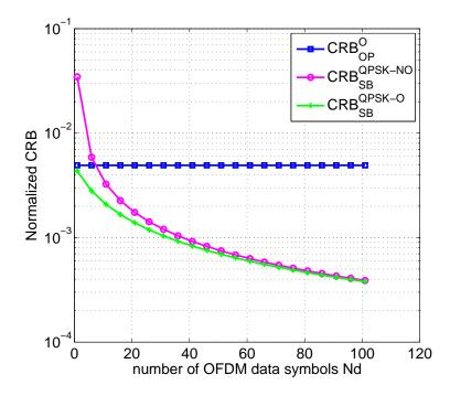
Figure 2.9: Normalized CRB versus number of OFDM data symbols  $N_d$ .
