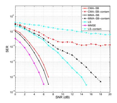
Figure 3.6: Average SER vs SNR under pilot contamination with asynchronous cells  $(N_r = 20, N_t = 2 \text{ per cell}, N_c = 4, N_d = 100, N_p = 5)$
