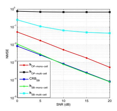
Figure 2.12: NMSE of LS and LS-DF estimators versus SNR with small inter-cell delays
