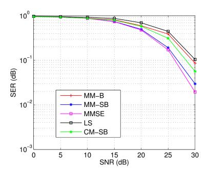
$\textbf{Figure 3.10:} \ SER \ vs \ SNR \ with \ 64\text{-}QAM \ (MIMO\text{-}OFDM \ model).$
