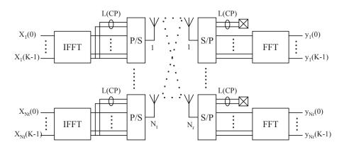
Figure 2.2: MIMO-OFDM communications system.
