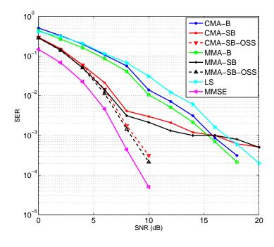
Figure 3.2: Average SER vs SNR for blind and semi-blind source separation with pilot-based initialization  $(N_r = 20, N_t = 4, N_d = 100, N_p = 5)$
