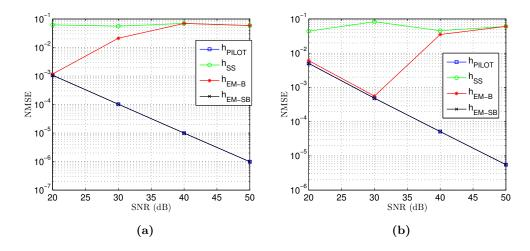
Figure 5.9: NMSE vs. SNR with  $M_L = 4$  and  $M_{NL} = 2$  for subspace-based estimator  $(h_{SS})$ , blind  $(h_{EM-B})$  and semi-blind  $(h_{EM-SB})$  EM-based estimators benchmarked against the fully-pilot-based estimator  $(h_{PILOT})$ . We consider: (a) quadratic model and 4-QAM modulation, and (b) cubic model and 16-QAM modulation.
