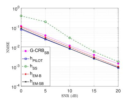
**Figure 5.7:** NMSE vs. SNR for subspace-based estimator  $(h_{SS})$ , blind  $(h_{EM-B})$  and semi-blind  $(h_{EM-SB})$  EM-based estimators benchmarked against the semi-blind Gaussian CRB (G-CRB<sub>SB</sub>) and the fully-pilot-based estimator  $(h_{PILOT})$ , in the case of a quadratic model, 4-QAM modulation and  $N_r = 9$  receive antennas.
