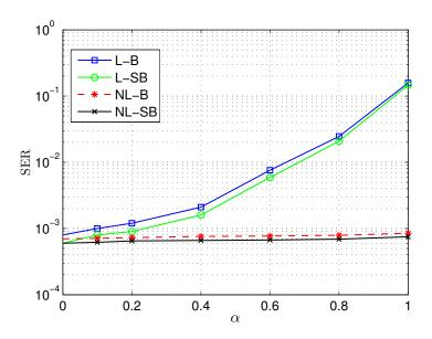
**Figure 5.4:** SER vs.  $\alpha$  with SNR = 5 dB for linear blind and semi-blind (L-B, L-SB) EM-based estimators and for nonlinear (NL-B, NL-SB) ones.
