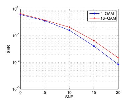
**Figure 6.7:** SER v.s. SNR for 4-QAM and 16-QAM constellations, with  $N_t = 2, N_r = 2$  and 5-th order nonlinear model.
