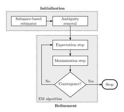
Figure 5.1: Proposed blind channel estimation scheme.
