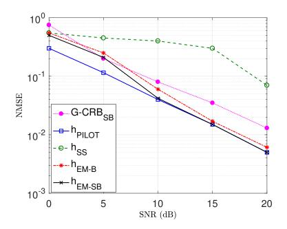
**Figure 5.8:** NMSE vs. SNR for subspace-based estimator  $(h_{SS})$ , blind  $(h_{EM-B})$  and semi-blind  $(h_{EM-SB})$  EM-based estimators benchmarked against the semi-blind Gaussian CRB (G-CRB<sub>SB</sub>) and the fully-pilot-based estimator  $(h_{PILOT})$ . We consider a cubic model and 16-QAM modulation.
