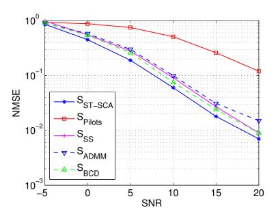
Figure 4.2: NMSE of data matrix S estimate vs. SNR.
