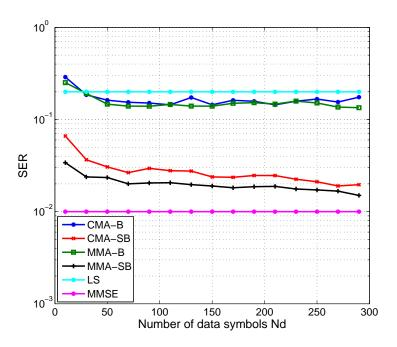
Figure 3.5: Average SER vs number of data symbols  $N_d$  for blind and semi-blind source separation  $(N_r = 20, N_t = 4, N_p = 5, SNR = 5dB)$
