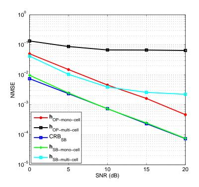
Figure 2.13: NMSE of LS and LS-DF estimators versus SNR with large inter-cell delays.
