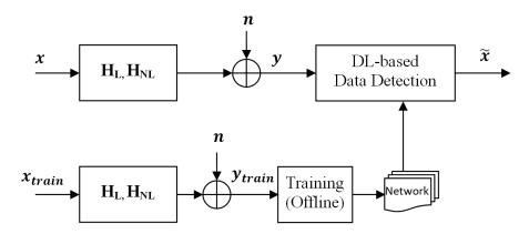
Figure 6.1: DL based data detection.
