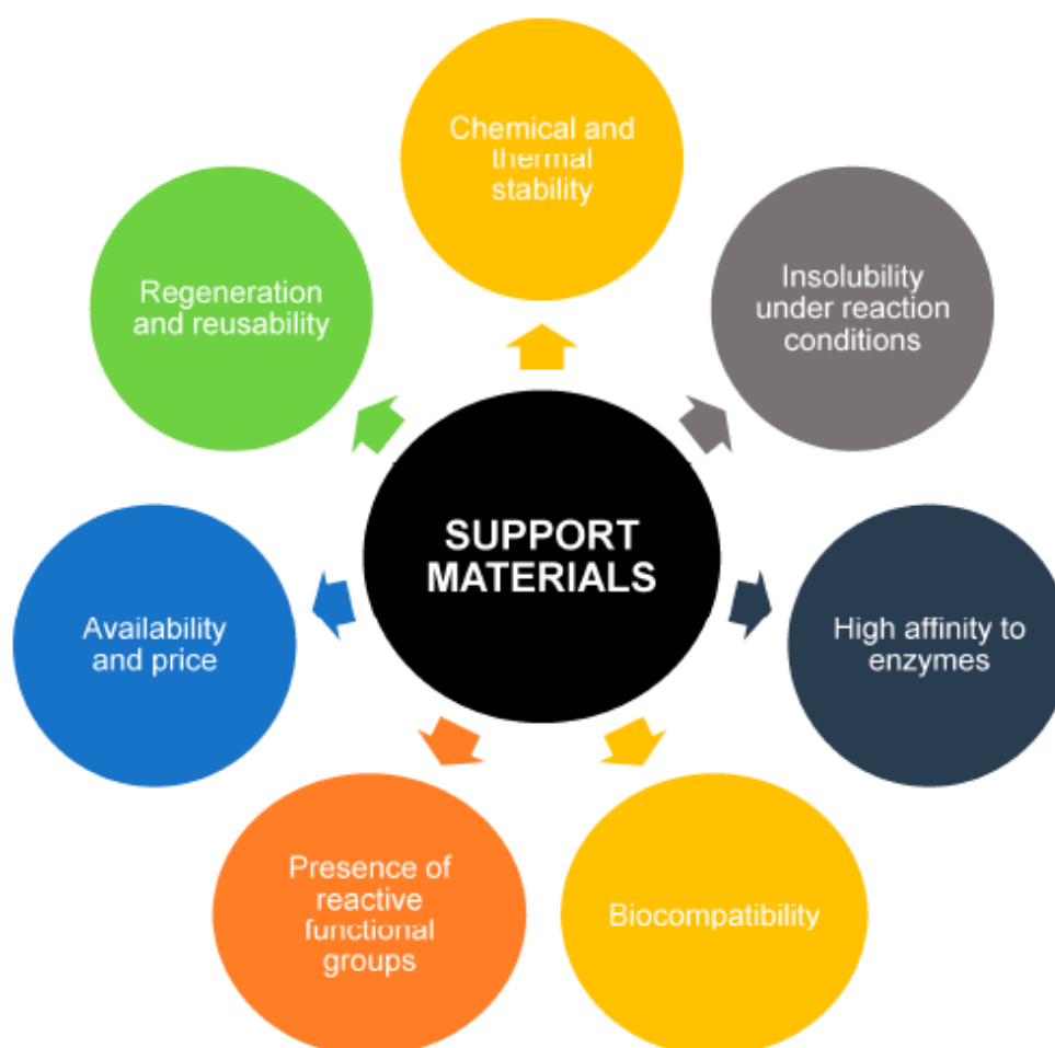
Figure 1.9. – Main features of support materials required for effective enzyme immobilization (Zdarta et al., 2018).
