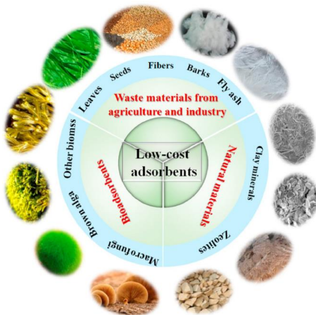
Figure 1.2. – The common low-cost adsorbents for the removal of dyes from aqueous solution (Siddiqui et al., 2019).
