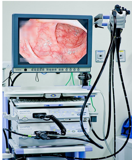
Figure 3.7: Monitor machine to which the endoscope in Figure 3.6 is related in order to transmit the images of the colon.
