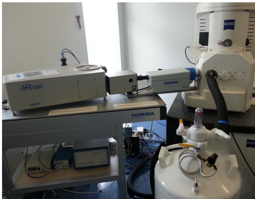
Figure II.18 - CL spectrometer picture available at LSPM. A liquid nitrogen bottle is used to decrease the temperature to 80K.
