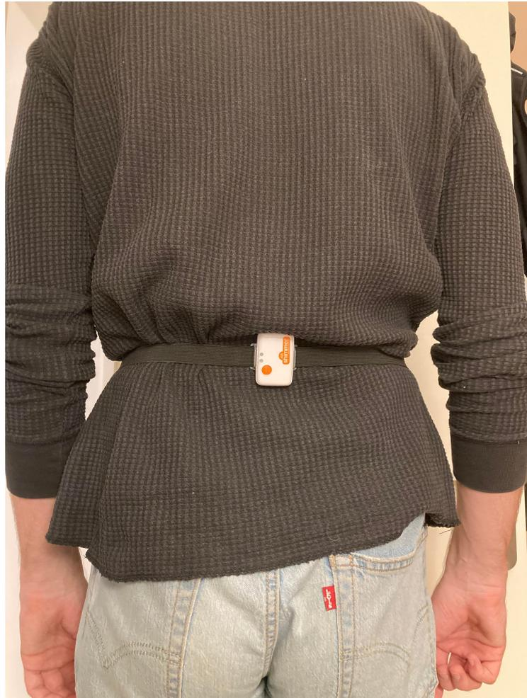
Figure 3.3: Inertial sensor location used for implemented protocols
