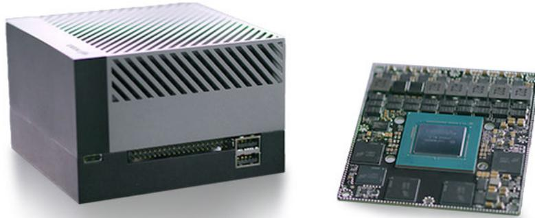
Figure 9.2: Nvidia AGX Orin, development kit (left) and production (right) GPUs.
