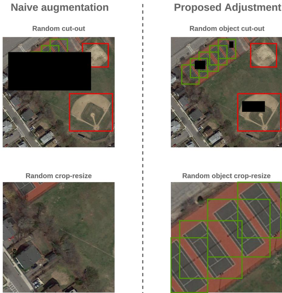
Figure 6.3: Difference between naive augmentation techniques (left) and our adaptation to object detection (right). The proposed transformations are applied at the object-level to preserve objects integrity.
