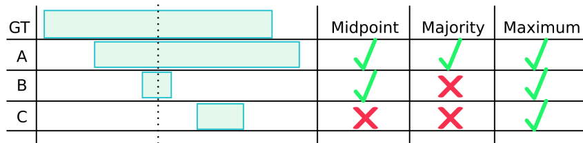
Figure 5.2: Common decision functions for the correctness of an event, such as midpoint, majority, and maximum. The horizontal rows represent the ground truth and different predictions. The vertical dashed line represents the midpoint of the ground truth.
