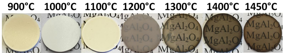
Figure 4.15: Photographs of Sasol MAS ceramics SPSed for 20 min at different temperatures between 900 and 1450°C
