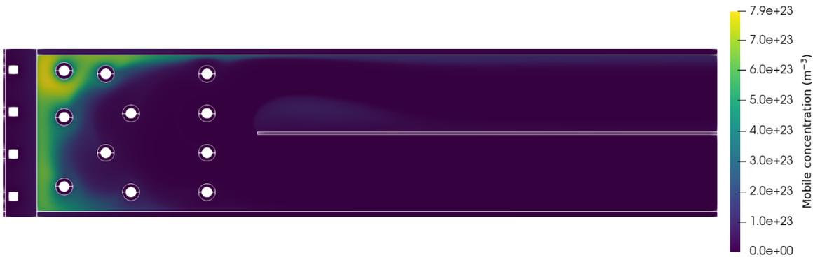
Figure 3.13: Tritium mobile concentration,  $c_m$ , field at steady-state
