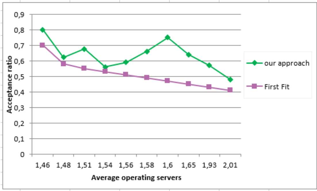
Figure 3.12: comparison of SFC request acceptance ratio between our approach and First Fit algorithm
