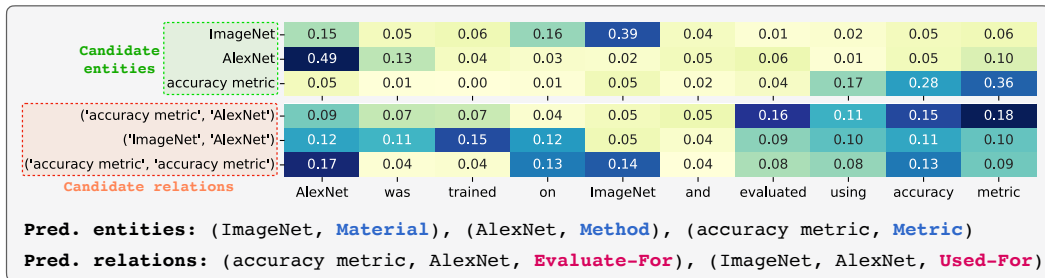
Figure 9.4: Attention visualization. This illustrates the attention score of candidate entities and candidate relations with the input sequence, averaged across attention heads.
